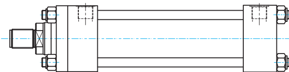
CD - DK series standard tie-rods hydraulic cylinder.
